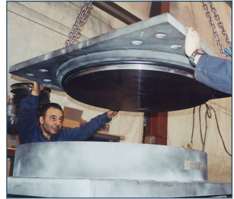
26,000 kN Pot Bearing Capacity Jacksonville & Syracuse Tower U.S.A.
