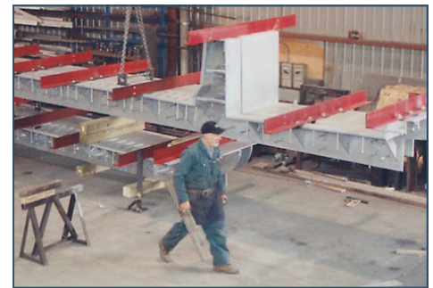
58 Feet Long Finger Expansion Joint Highway 4 Over North Saskatchewan River Saskatchewan, Canada
